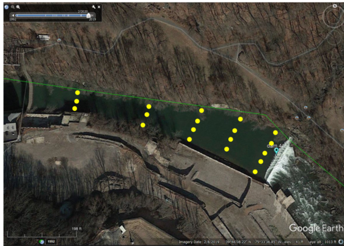
Dam 4 Sediment Analysis Transects
